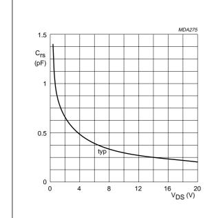
Fig.2  $V_{GS}$  = 0 for BF510 and BF511;  $I_D$  = 5 mA for BF512 and BF513; f = 1 MHz;  $T_{amb}$  = 25 °C.
